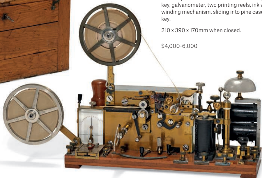
62 TELEGRAPHY - A cased telegraph manufactured by L.M. Ericcson & Co., Stockholm, c.1890.
